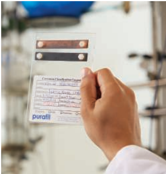
FIGURE 3. Corrosion classification coupons (CCCs) are used to establish baseline corrosion data
