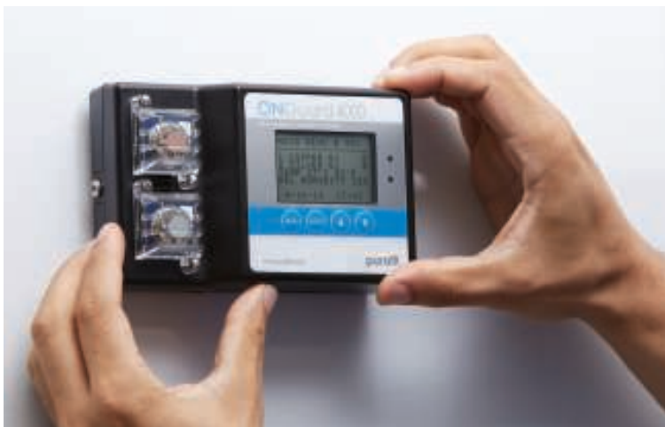
FIGURE 4. Atmospheric corrosion monitors (ACMs) provide realtime data on the performance of the corrosion-prevention measures in a control room, including chemical-filtration and air-quality systems
