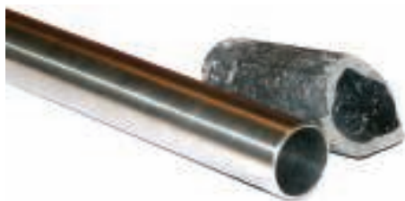
FIGURE 4. A high-chromium alloy austenitic stainless steel tube (left) pictured alongside standard graphite tube (right).
