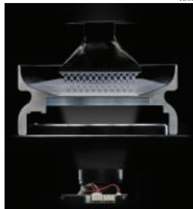
FIGURE 1. Carbon’s CLIP process addresses speed and finish issues in 3-D printing of final parts
